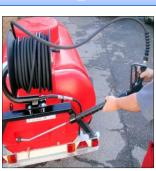
Remove lance from holder and pull hose off to desired length
