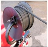
Replace the pin to lock the hose reel in place and begin work.
