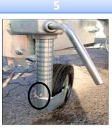
Turn jockey wheel clamp anti-clockwise until pin in place with U
