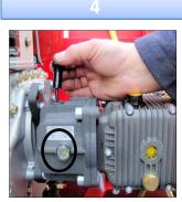
Check the oil in the gear box – using dipstick or sight level
