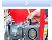
Check the oil in the pump – using dipstick or sight level
