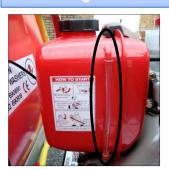
Check diesel using sight level and fill as required.
