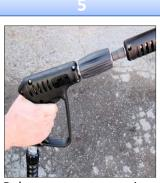
Release any pressure in the hose by squeezing the trigger.
