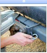
Attach to tow bar ring if possible or back around safety brake cable.
