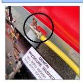
Check ball valve is in the 'on' position.
