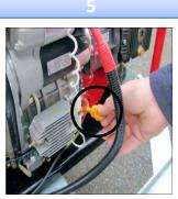
Check the engine oil. Replenish as required.
