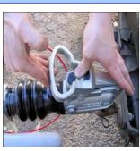
Hold up bowser handle, push button and lift hitch to release lock.
