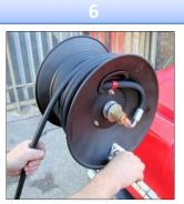
Release pin on hose reel and wind hose in and replace pin.
