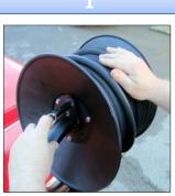
Pull pin on hose reel to release hose.
