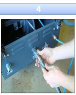
Connect to mains water by pulling back inlet and pushing hose on.
