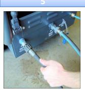
Connect MVG High pressure hose. Push I MVG nipple & tighten nut
