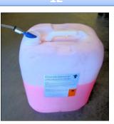
For detergent. Insert detergent pipe into chemical drum.
