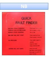
For faults refer to the instruction panel on the front right hand side of the machine prior to calling for technical assistance.
