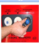
Ensure hot water on. Adjust detergent valve accordingly.
