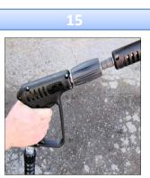
Release any pressure in hose by squeezing trigger and disconnect.
