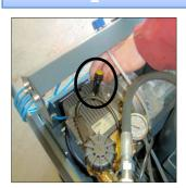
Unlock bonnet clips, lift lid and check pump oil. Replenish as required.
