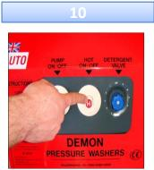
For hot water push button and hot water will filter through.
