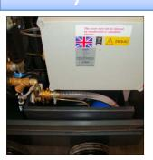
Turn on mains water. Water tank will begin to fill inside machine.
