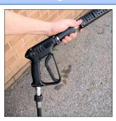
Connect hose to trigger – ensure correct lance for hot water is used.
