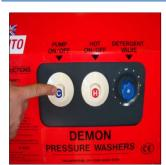
Shut down lid and push button to turn pump on to get cold water.
